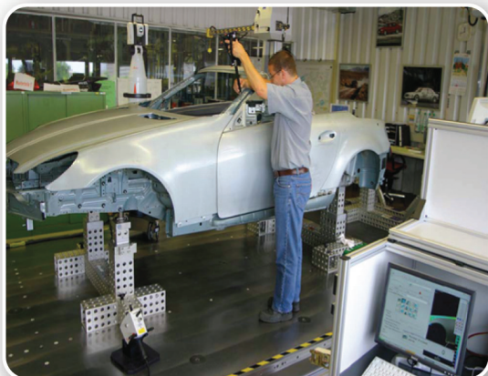
Random inspection of control points of a body in white for statistical purposes and trend monitoring. T-Probe and T-San are used for this task. Automated analysis including reporting is achieved by using macros.
