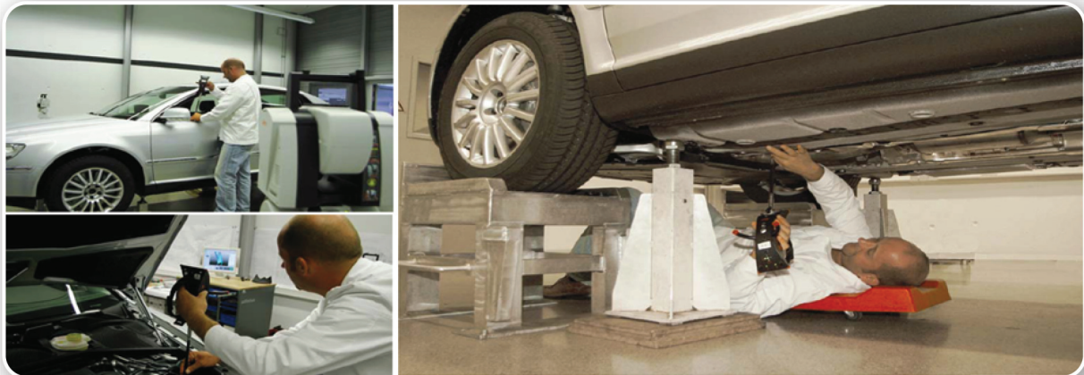
Final geometry checks for trend monitoring. Detected deviation trends are corrected in the production and assembly lines.
